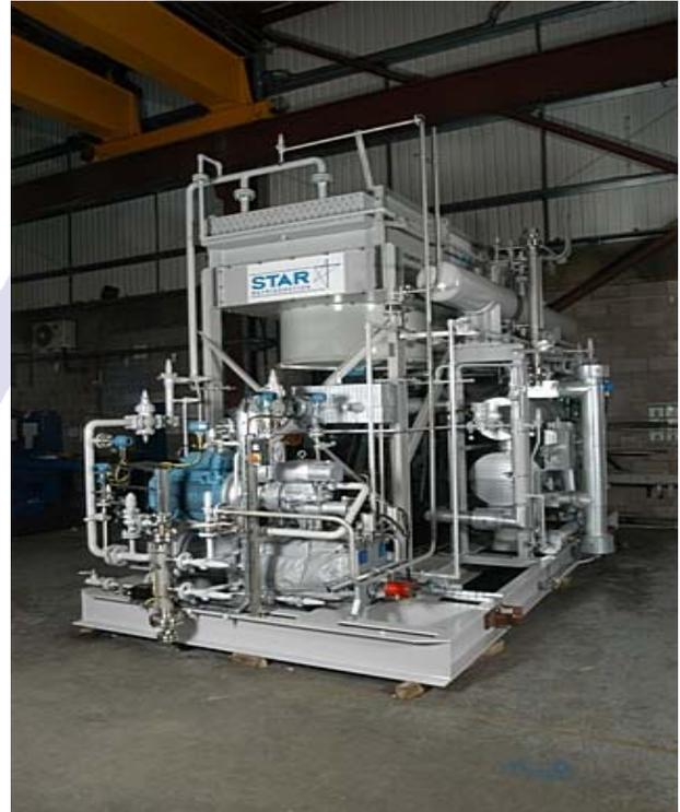
The package consisted of an oil injected screw compressor, close coupled Zone 2 Ex N drive motor, API 661 compliant air-cooled condenser, liquid receiver and shell & tube evaporator with all interconnecting pipe work and package unit wiring terminating at package junction boxes and skid mounted Control Panel.
