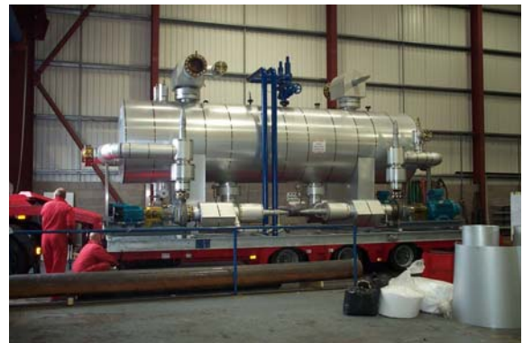
Complete tank/pump skid with latent heat storage tank, Therminol expansion tank and process pumps
