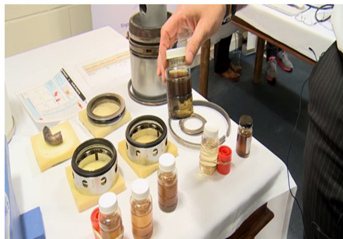
An oil sample should be taken once a month to maintain the system at its correct operating conditions
