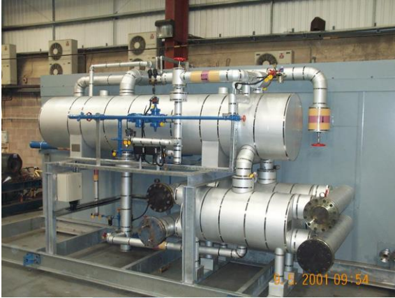
Star's custom built package including two Howden screw compressors, drive motors with acoustic enclosure, surge drum and two Vahterus plate and shell evaporators.
