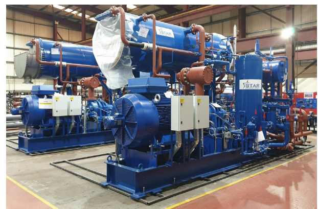
Twin Water Source Heat Pump for Queens Quay
