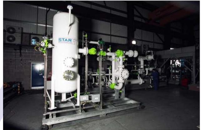
Interconnecting Site Pipe work was provided and the refrigeration plant controlled from a remote mounted Allen Bradley PLC. The complete system is suitable for operation outdoors within a Hazardous Zone 2 IIB T3 Area environment.
