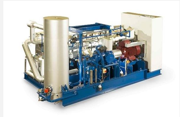
Ramsund's **Neatpump** was built at Star's Glasgow manufacturing facility and was shipped as a complete packaged unit, ready for installation in an existing plant room at the military base. The plant has a 600kW capacity and a COP (Coefficient of Performance) of 2.7, heating water to temperatures between 60 and 68 degrees Celsius.
